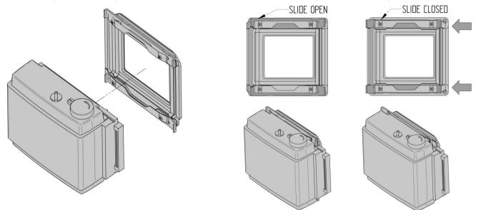
Please mount the roll film holder to the WRS-1068 adapter before mounting the adapter to the Cambo WRS. Be for mounting the roll film holder ensure that the slides of the adapter are fully opened. Place the holder (only fits one way) and close both slides to lock the holder in place.
